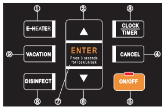
**Note:** Pressing any key will have no effect, unless the keylock is disabled on the control interface.
