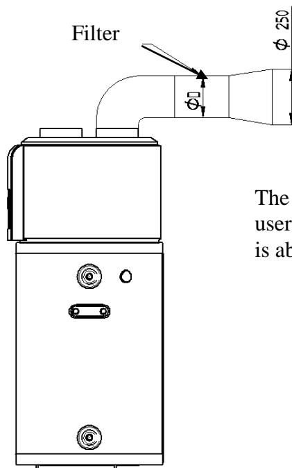
The filter must be mounted by the user of the appliance, the mesh size is about 1.2mm.
