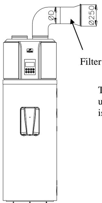
The filter must be mounted by the user of the appliance, the mesh size is about 1.2mm.
